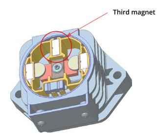
Non polarised contactors use a third magnet to move the arc away. This is why non polarised contactors are a little more expensive.
