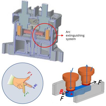
I = Current direction, B = Magnet field, F = direction of movement (of the arc)
