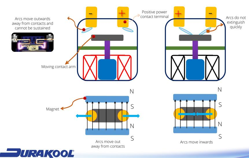
In the left drawing, you can see how the arcs are pushed away from the moving contacts.
